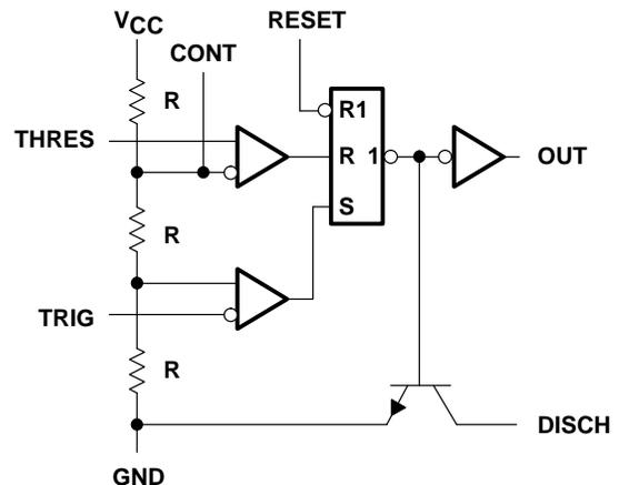
RESET can override TRIG, which can override THRES.
