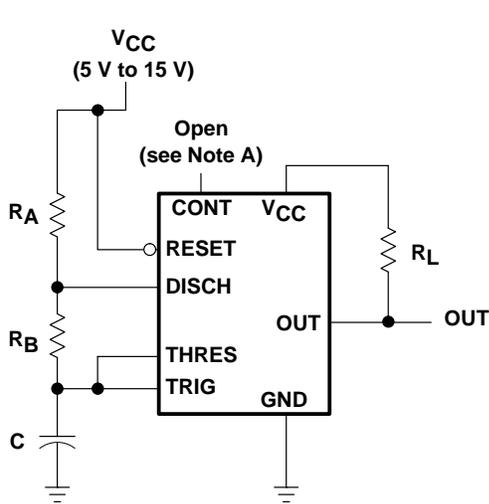
NOTE A: Bypassing the control voltage input to ground with a capacitor may improve operation. This should be evaluated for individual applications.
